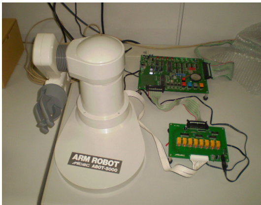
Fig. 1 Robot arm with four DC motors.
