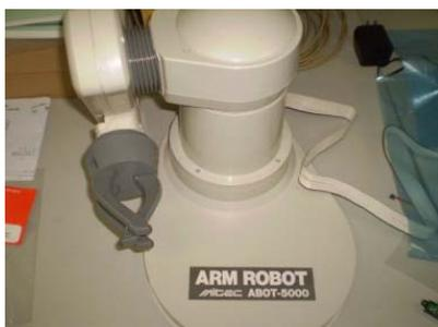
Fig. 1 Robot arm with 4-DOF
