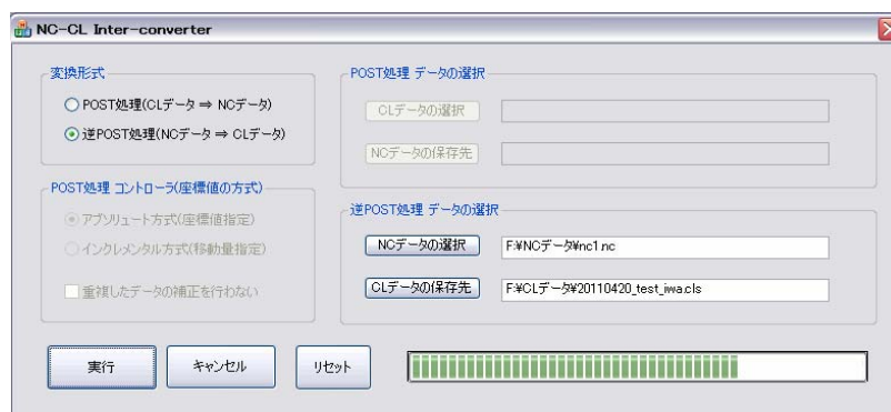
Fig. 1 Reverse post-processor from NC data to CL data.
